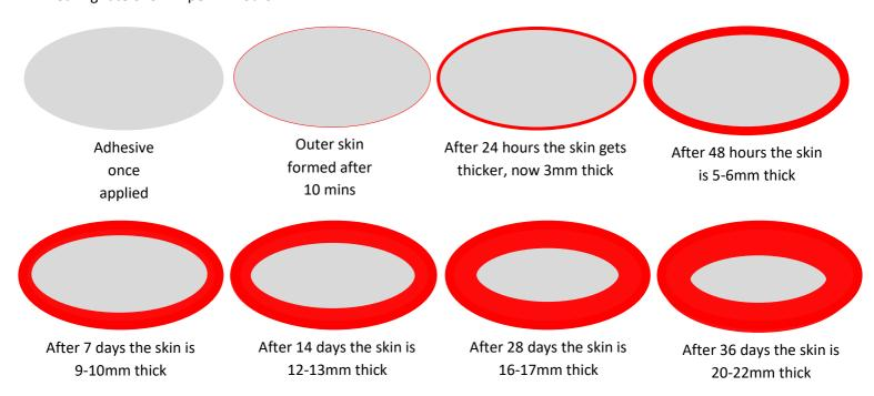
As shown above, over time the adhesive will eventually cure, but as the moisture needs to travel through the outer skin and as this skin gets thicker, the curing rate per 24 hours reduces. If the 2 substrates were separated prior to the full cure of the adhesive, then the adhesive in the centre will still be wet.
