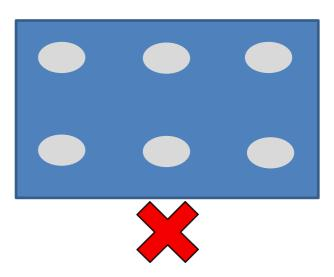
When a moisture cure adhesive is applied in beads, the adhesive will reach full cure 5-10 times faster than daubs as the moisture from the air needs to go through the cured adhesive and reach the centre.
