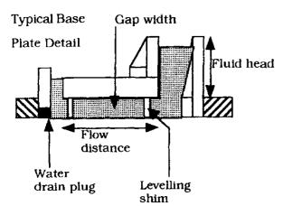
Pouring should be from one side of the void to eliminate any air or presoaking water from being trapped under the baseplate.
